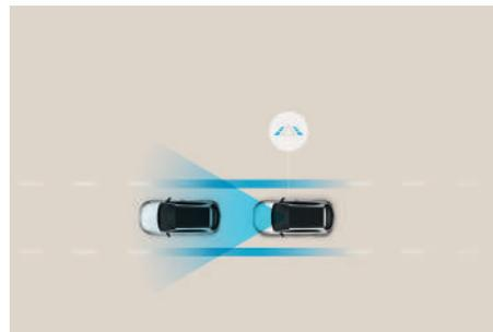
**Lane Follow Assist (LFA):** Smart sensors and the forward-facing camera detect when the car drifts from the centre of the lane, applying steering torque to hold road positioning for safety. The car also estimates the trajectory of the vehicle ahead and adjusts its position accordingly.
