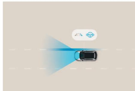
**Lane Keep Assist (LKA):** The Lane Keep Assist (LKA) uses the front multi-function camera to monitor the lines of the road. In case of an unintended lane departure, it warns you and can apply counter steering torque to guide the car back to the lane.
