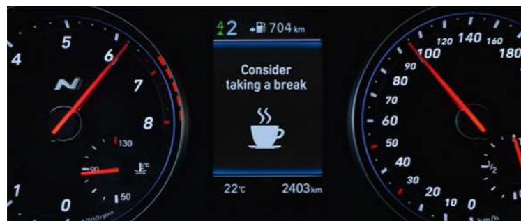
Driver Attention Alert (DAA): This standard feature raises safety and convenience to an entirely new level by continuously monitoring and analysing driving patterns. When a pattern of fatigue or distraction is identified, DAA gets the driver's attention with an audible alert and pop-up message suggesting a break.
