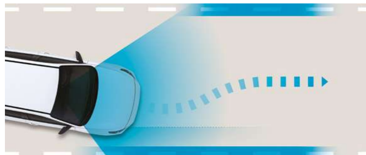
Lane Keeping Assist (LKA): At speeds over 37 mph the system alerts the driver about unsafe movements. In case of an unintended lane departure, it will warn the driver and can apply counter steering torque to guide the car back to a safe position.
