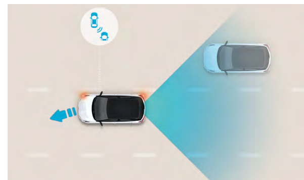
Blind Spot Collision Avoidance Assist (BCA): Radars detect traffic in the vehicle blind spot, warning drivers with an audible alarm when the indicator is used so you can be aware of the traffic around you. It will also take action itself, braking to help avoid a collision. Standard on Premium and Ultimate trims.
